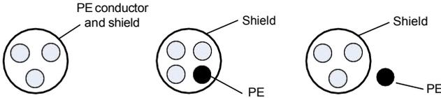
To suppress emission and conduction of the radio frequency interference effectively, the shield of the shielded cable is copper braid. The braided density of the cooper braid should be greater than 90% to enhance the shielding efficiency and conductivity, as shown in the following figure.
