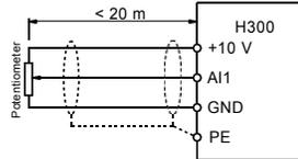
In applications where the analog signal suffers severe interference, install filter capacitor or ferrite magnetic core at the analog signal source.
