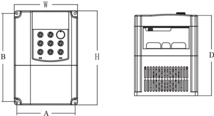
Figure 8-2 Physical appearance and overall dimensions of the H300 (sheet metal housing)
