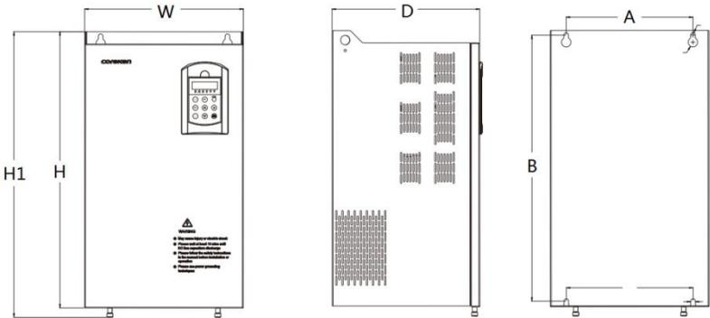
Table 8-2 Overall dimensions and mounting hole dimensions of the H300
